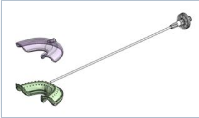
FIG 1A: The two halves of the mouth dispenser before solvent bonding along with the input tubing.
